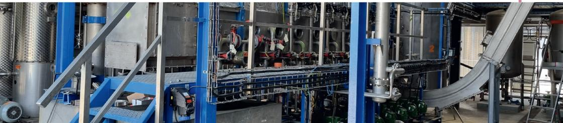
The GAIA project led by Exinnov aims to develop plant extraction using biobased solvents. Adapting equipment previously used with hexane has enabled the commissioning of an industrial continuous countercurrent extractor that can withstand the constraints of 2-methyloxolane, a green solvent produced from by-products from the agri-food industry.
